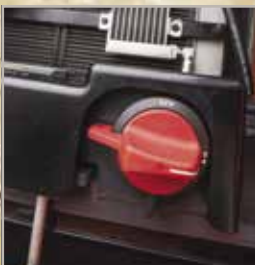
Battery cut-off switch
