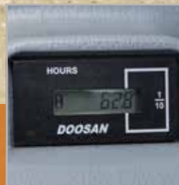
Hour meter (from ground level)
