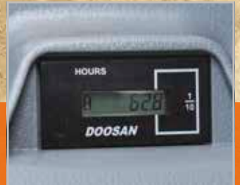
Hour meter (from ground level)
