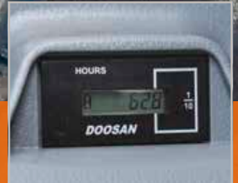
Hour meter (from ground level)
