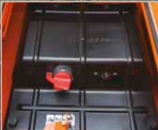
Battery cut-off switch
