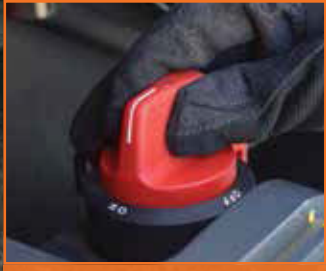
Battery cut-off switch
