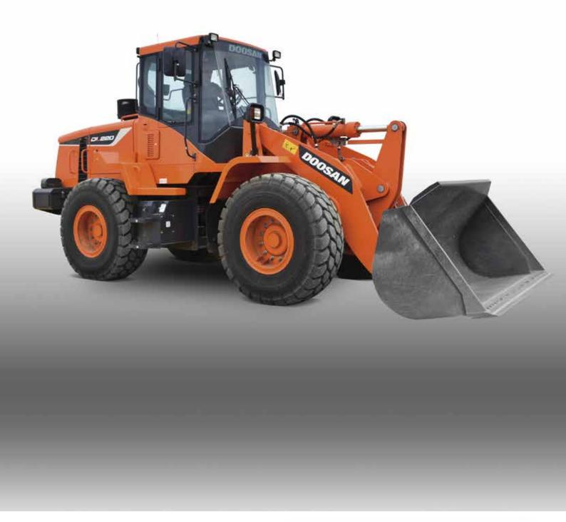
Maximum power: 160 hp Operating weight: 12365 kg Bucket capacity: 2.2 m³
